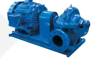
Model 411 is horizontally baseplate mounted with a driver flexibly coupled to the pump. This design is recommended where floor space is readily available and where flooding of the installation is not possible.
